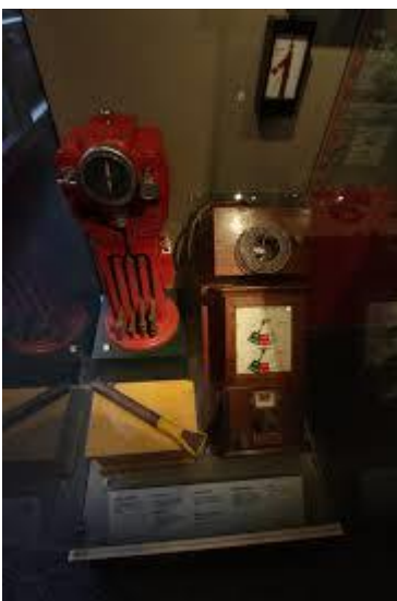
These miniatures show left to right: Staff Instrument, Block Instrument, and a Staff Box in the foreground.
