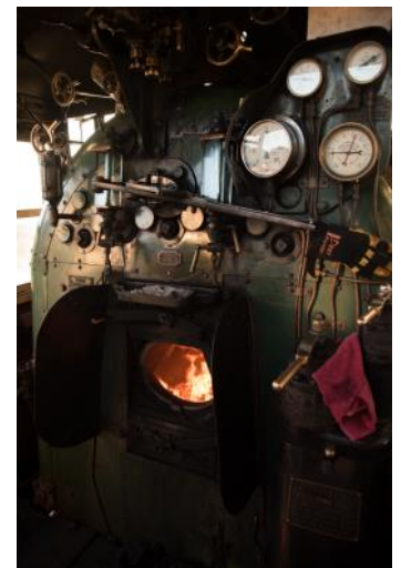
Fire Box on the Steam Train Visiting Townville 12 June 2017.
